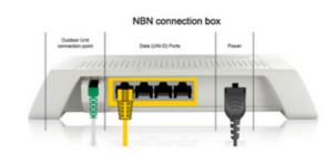
Using an ethernet network cable connect your router from its WAN port to the relevant Uni-D port on the NBN Connection Box. We generally activate the next available Uni-D port – starting with Uni-D 1. We will detail your Uni-D port number in our emails to you.
